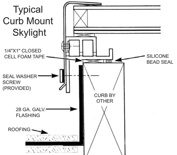
**5 Flashing the curb.** Install flashing as illustrated, up the curb to make a neat tight fit. Tack flashing to curb as necessary. One piece head & tail wrap around and seals corners of curb. Underlay shingles with flashing as roofing is built up along the sides of the curb. See steps 1-4 above.
