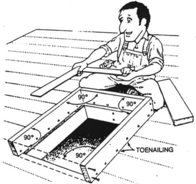
**4 Building the curb.** Using 2" x 4" to 2" x 12" lumber build a rectangular frame - or curb - mounted flush with the opening. All corners must be 90 degrees. Check to see if your skylite fits the curb. The top of the curb must be flush with the underside of the skylite. Remove unit and proceed to the next step.
