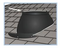
**STEP 17** - If there is excess light pipe **(G)** sticking out of the flashing, using tin snips, cut from the top down to the lip of the flashing and trim off the excess pipe.
