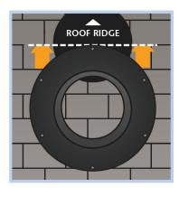
STEP 11 - Apply caulk over all exposed screw heads (since they will be exposed to the weather). Use remaining caulk to seal the areas where the 4" slits were made and around area where shingles meet with raised area of the flashing.
