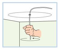
Mark the center of the ceiling ring (K), drill a hole and insert a piece of wire bent at a 90 degree angle. Rotate the wire around 360 degrees. While rotating, feel for resistance that could indicate wire runs or other obstructions.
