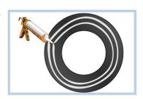
STEP 10 - Taking care not to smear caulk on the exposed shingles, slide the flashing under the tar paper and shingles and force flashing up until the shingles come in contact with the raised portion of the flashing. The bottom side of the flashing will be on top of the shingles. Secure flashing with six Phillips head screws (D).
