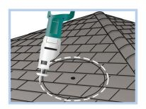
**STEP 7** - With a utility knife, cut a four inch slit through the shingles and tar paper at the 3 and 9 o'clock positions of the flashing. This allows for the footprint of the flashing to be inserted under the shingles.
