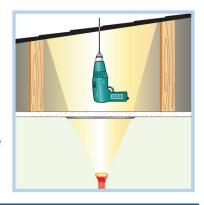
STEP 5 - On the roof, locate the centering hole and outline the diameter of the hole that the pipe will pass through by turning the flashing (E) upside down and marking the inside of the flashing unit.
