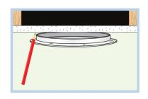
STEP 3 - Install the ceiling ring (K) on the ceiling. Place ceiling ring in the hole cut in Step 2. Peel the protective covering off the white horsehair gasket (H) and apply gasket to the inner lip of the ceiling ring (K). This gasket ensures a dust free fit
