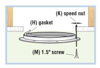
between the light pipe and the ceiling collar. Secure the ceiling collar to ceiling by inserting a 1 1/2" Phillips flathead screw (L) into one of the three pre-drilled dimpled holes and inserting it up through the drywall into speed nut (J) provided. Repeat this process for the other two screws.
